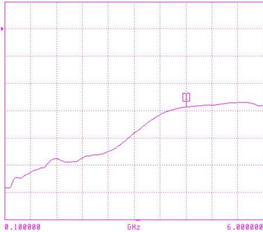
Figure 5 Isolation Common to Inactive Port
