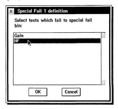
Select [highlight] the **Data Name(s)** for the test limit check(s) you want to designated as a Special Fail Limit Check for the special fail category selected. (The Data Names selected will be reverse highlighted by the System Computer.)
