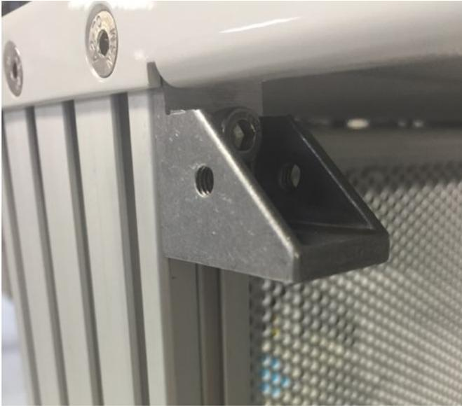
After the panel is removed, add the triangle bracket to the left or right metal extrusion upright (as shown in Figure 2) using the M5 x 22 mm Cap Head Screw (MGSUBS1A) and M4 Allen Wrench. Left mounted triangle bracket is for a right offset tray, and right mounted triangle bracket is for a left offset tray.
