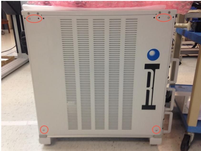
Figure 1: Removing the cover screws. (Left mounted Tray)
