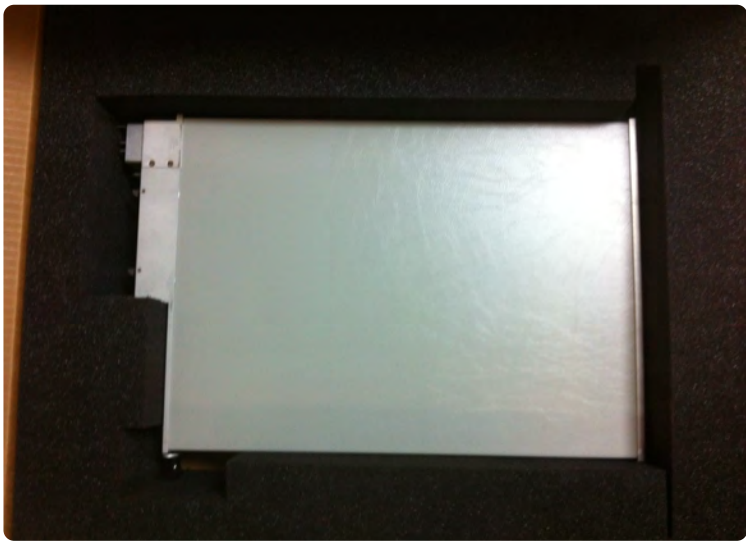
FIGURE 1.47 TIM PLACEMENT IN SHIPPING CONTAINER
