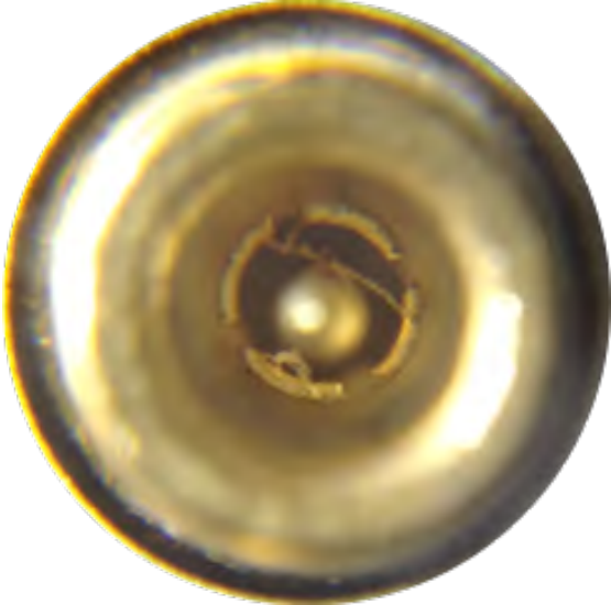
FIGURE 3.5 DIRTY PKZ #12 CONNECTOR EXAMPLE
