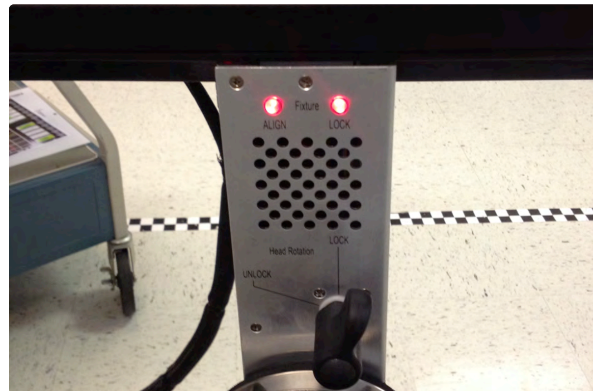
FIGURE 1.53 FIXTURE DOCKING INDICATOR LIGHTS
