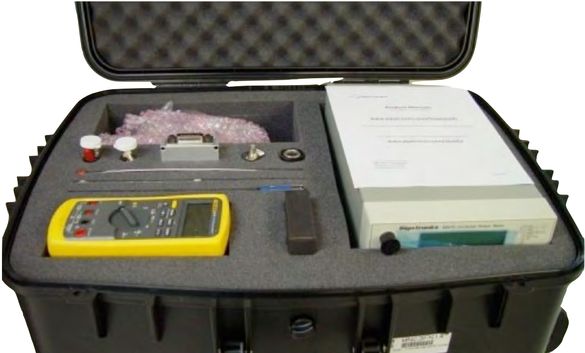
FIGURE 6.2 CALIBRATION KIT, 20 GHz
