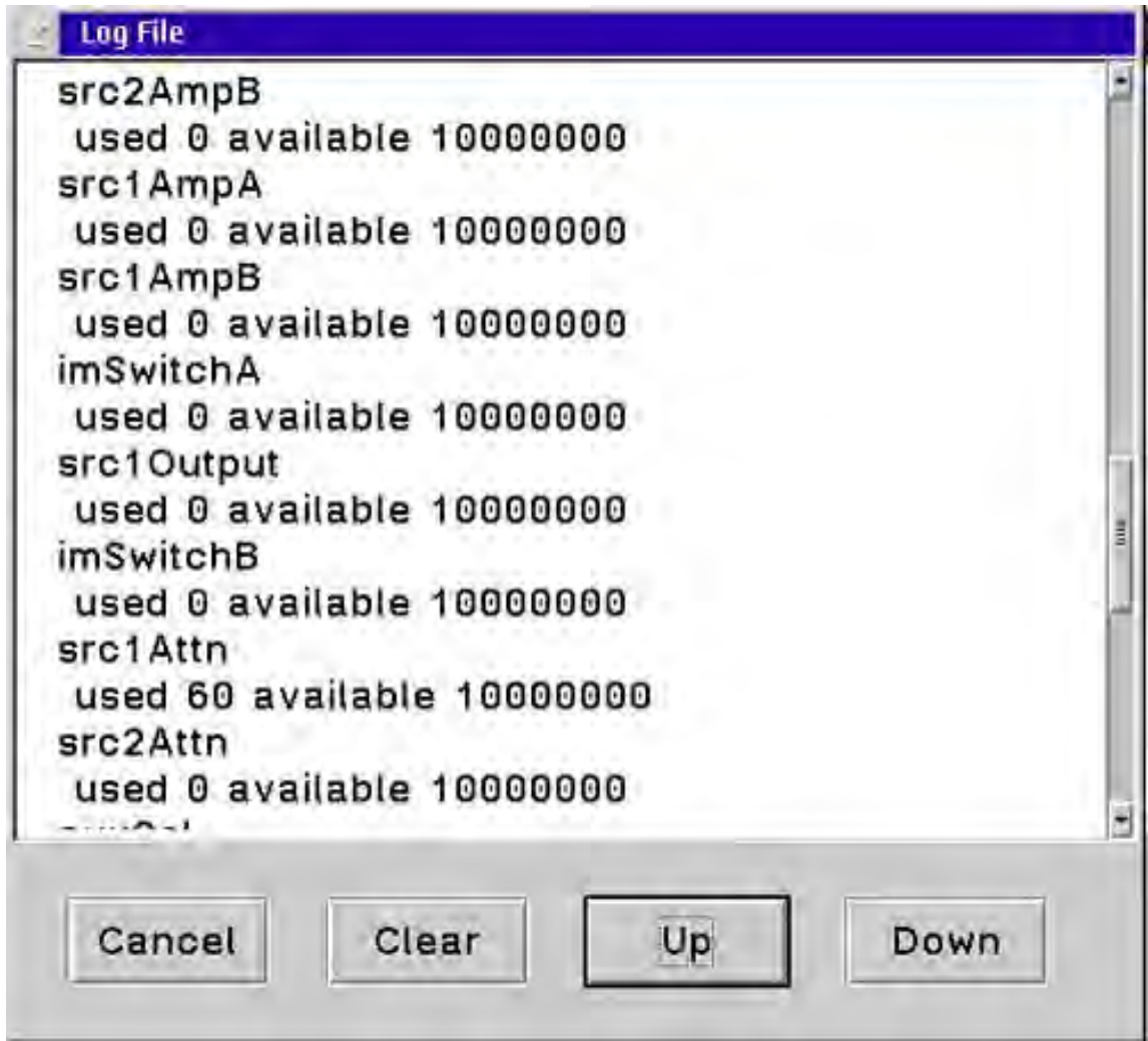
FIGURE 4.3 SWITCH WEAR LEVELS
