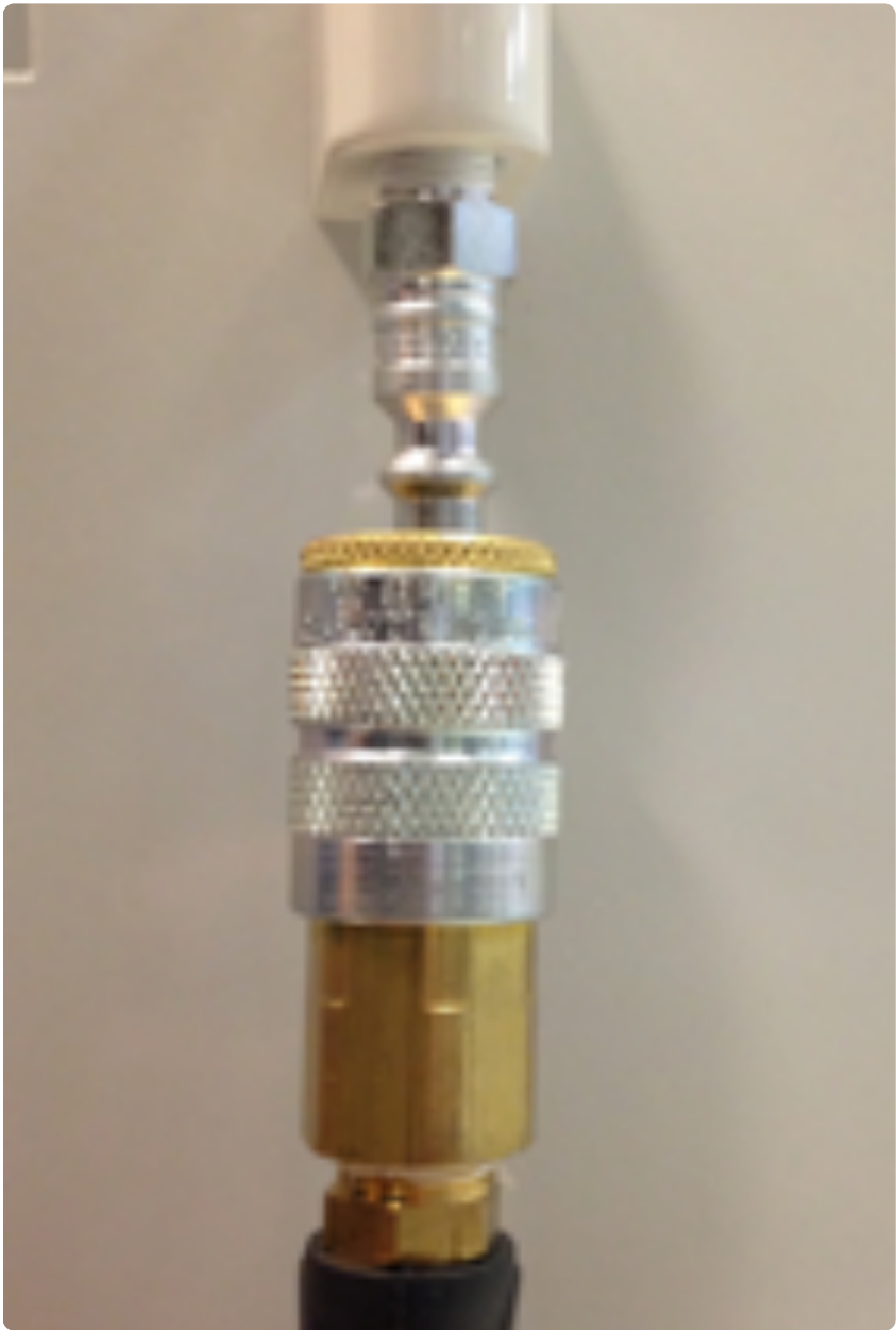
FIGURE 1.10 CORRECTLY INSTALLED NPT 0.25 IN FEMALE ADAPTER
