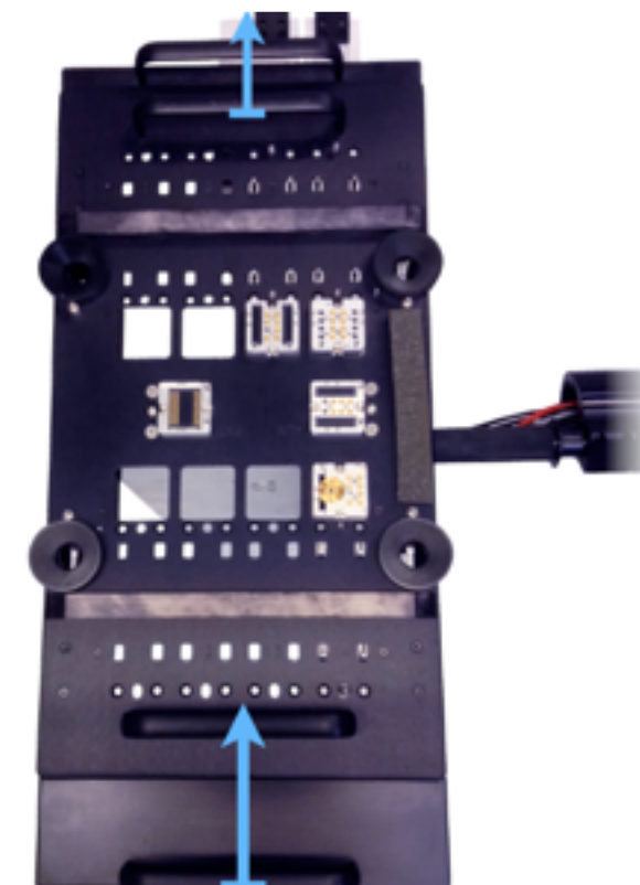
Actuation movement for locking a fixture to the test head.
