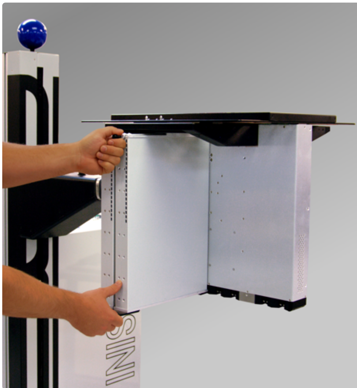
FIGURE 1.37 ADDING TIMS TO THE TEST HEAD
