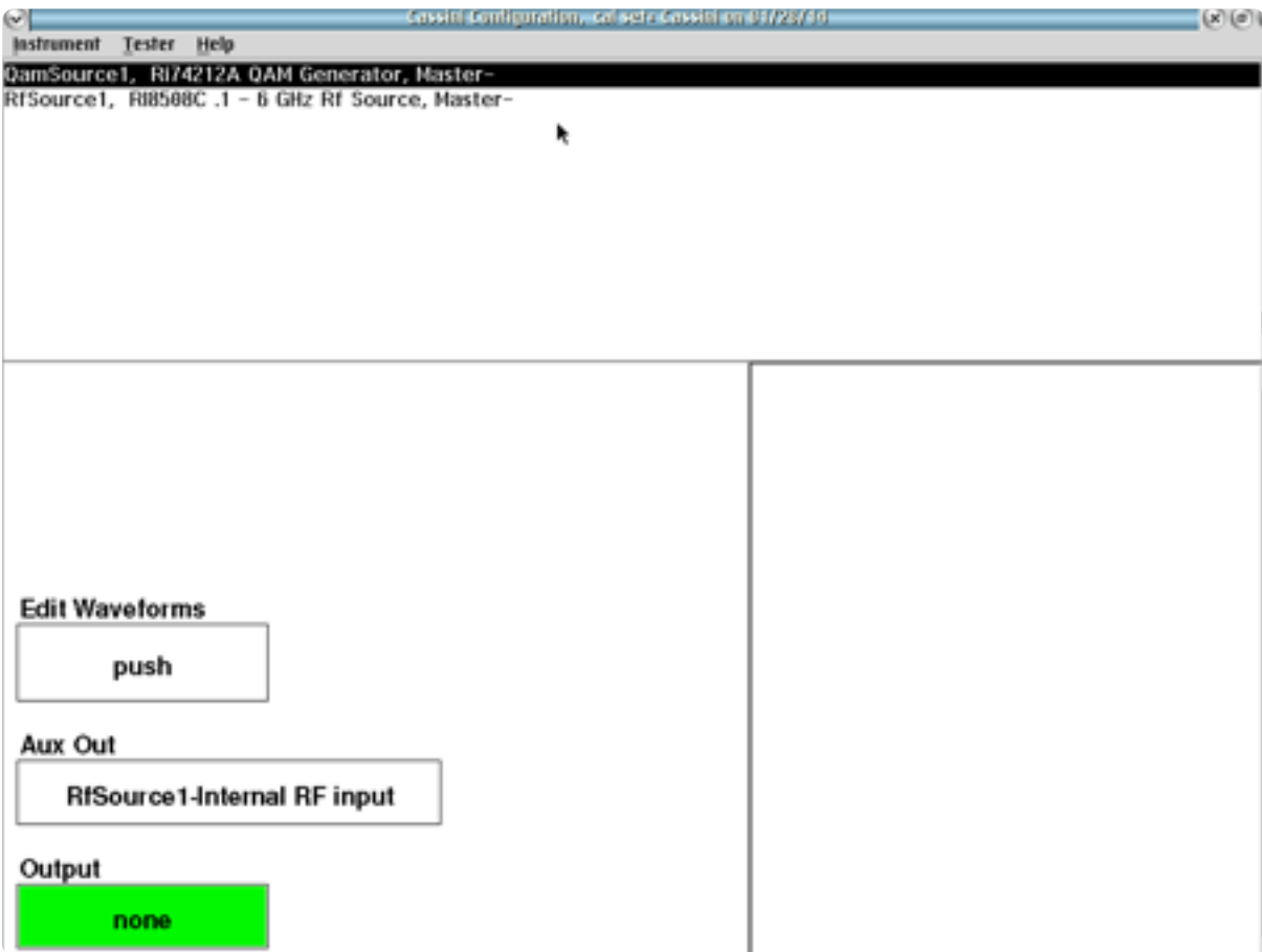
QamSource1 configurations including waveform and output configurations.
