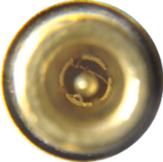
FIGURE 3.5 DIRTY PKZ #12 CONNECTOR EXAMPLE
