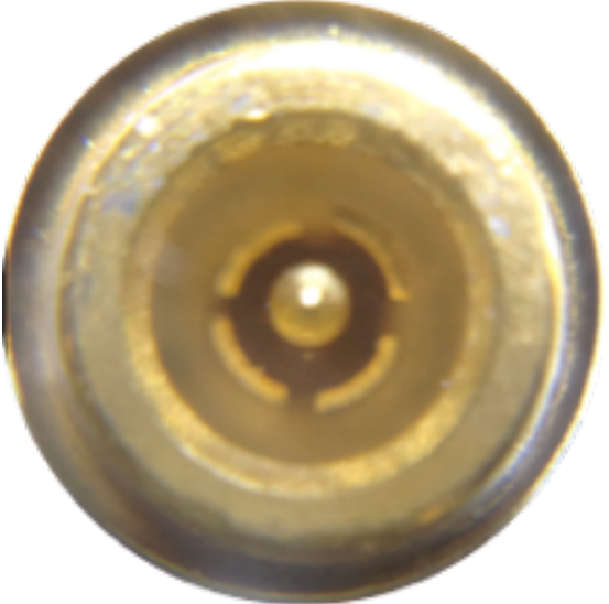
FIGURE 3.6 CLEAN PKZ #12 CONNECTOR EXAMPLE
