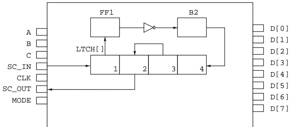
**Figure 3. Example device with scan hardware**
