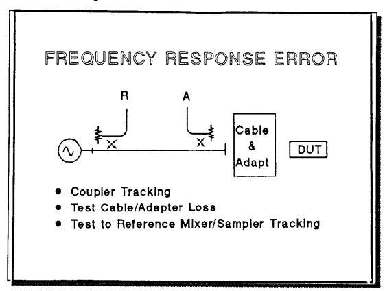
Reflection tracking errors are a composite of the frequency response of the couplers (coupler tracking), the test cables and the microwave mixer in the System Receiver.
