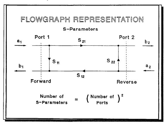
This is a flow graph representation of a two port device, such as the attenuator from the previous slide. The input port has two nodes: one representing the incident or **a** wave and one for the emerging **b** wave. Lines that connect nodes are called branches. Each branch has an arrow and a value corresponding to an S parameter. Energy will only flow in the direction of an arrow.
