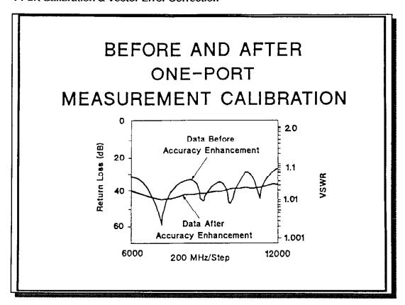
The impact of performing calibration and vector error correction to mathematically eliminate systematic errors (even for one port devices) is significant as you can see. The importance of vector error correction for multi port devices is even more critical.
