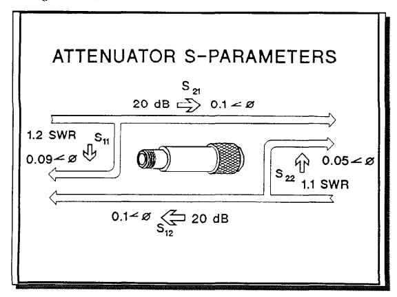
One of the advantages of S parameters is that they are intuitive. S21 is simply the forward gain or loss of the device in linear units. For the 20 dB attenuator shown, we see that the loss through the attenuator is equal to an S parameter voltage ratio of 0.1. Since S parameters are complex parameters, there is a phase angle term ( $\phi$ ) as well as a magnitude term associated with each S parameter. The SWR of the device is equivalent to the S11 or input voltage reflection coefficient of 0.09.
