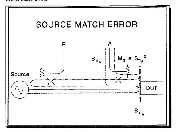
When a signal is reflected back off the test device into the test system, the signal does not see a ideal load due to all of the small mismatches errors caused by imperfect connections, transitions, etc. in the system. An error loop is formed with the signal bouncing back and forth (as shown in the slide.) This error is related to the product of mismatch terms and it is only a major factor when the test device has a large mismatch.
