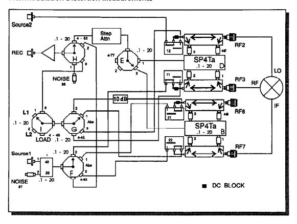
4 Port Test Configuration for Intermodulation Distortion of Mixers
