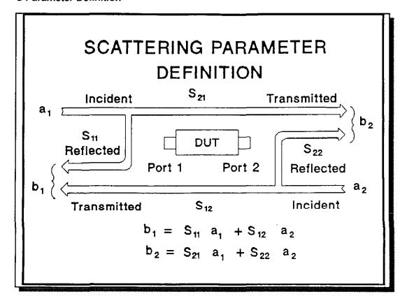
S parameters or Scattering parameters (S11, S12, S21, S22) define the relationship between the incident, transmitted and reflected signals at the inputs and outputs of the device under test. The examples and equations shown are for a 2 port RF device. a1, a2, b1 and b2 are defined below:
