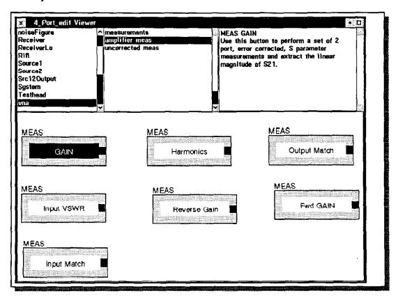
You create test plans, as previously shown, by copying buttons from other test plan panels (or from the Test Instrument Panels) and adding the buttons to a new test plan panel. For example to add the GAIN measurement button you select the **vna** instrument and the **amplifler meas** button types (shown above), select the **MEAS GAIN** button (highlight the button), and add the button to the test plan. The process takes just a few seconds. It is that simple and easy to create tests.
