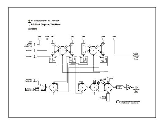
The RFICMMIC Test Head contains the couplers, microwave switches, Bi-state loads, the RFpower sensor and the noise source necessary to make multi-port S parameter, RF power and noise figure measurements.
