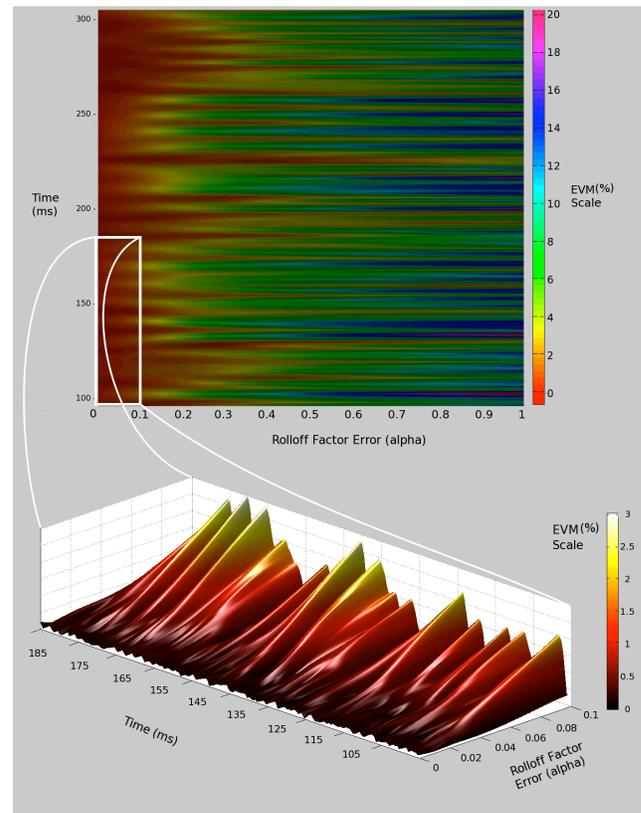
Fig. 4: (Upper Graph) Chromatogram showing variation in instantaneous EVM over time/recovered symbols (y-axis) versus mismatch error (x-axis); (Lower Graph) Zoomed-view of variations in EVM across 0 -0.1 Roll off Error
