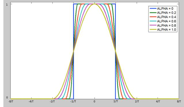
**Fig. 3: Frequency Response of Raised Cosine Filters with varying roll-off (alpha). Larger alpha relates to relaxed transition band roll off**
