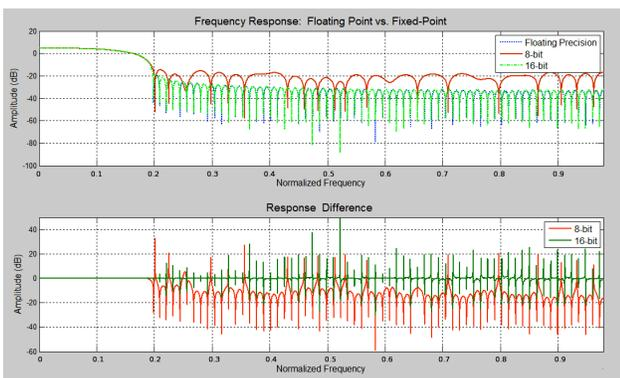
**Fig. 8: 8-bit and 16-bit Fixed-Point vs. Floating-point Precision Frequency Response (top) and corresponding differences (bottom)**
