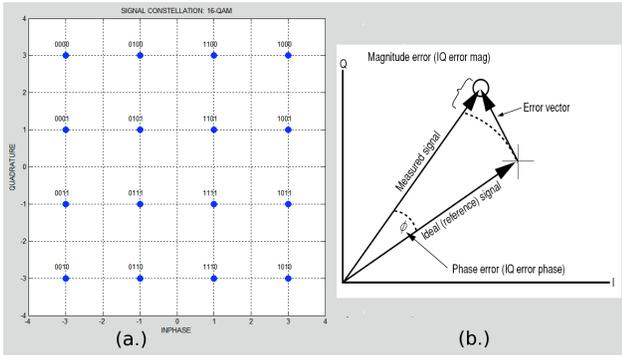
**Fig. 2: (a.) Example of a 16-QAM constellation and bit coding; (b.) vector representation of EVM and related components**
