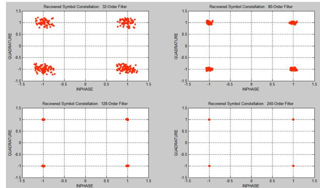
**Fig. 6: Recovered QPSK Symbol Constellations from Different Pulse-Shaping Filter Orders: 32-Order (top left); 80-Order (top right); 128-Order (bottom left); 240-Order (bottom right)**
