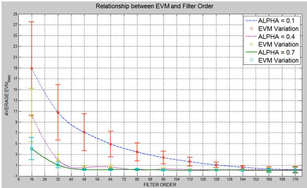
**Fig. 7: Relationship between EVM Error and Filter Order for roll-off values of: 0.1, 0.4, and 0.7**
