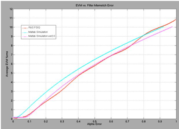
**Fig. 5: Comparison of Measured Average EVM from a R&S FSIQ (red) as a function of filter mismatch to simulation models (magenta; cyan) developed in MATLAB/Simulink. Version 2 plot is an offset of the original simulation used as a comparison reference**
