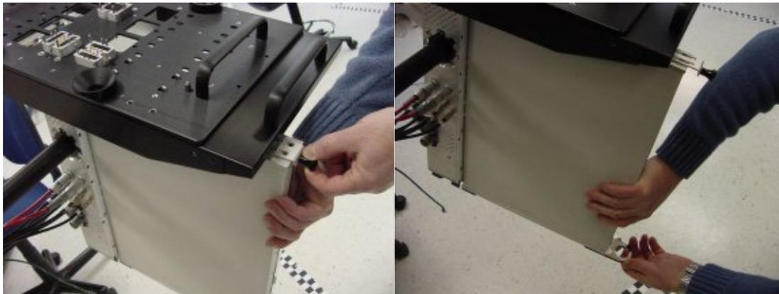
TIMs can be just as easily docked to the Testhead by sliding the module up into the slot until you hear it click. Then push in the top handle to power up the modules.
